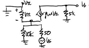
$$V_{TC} = -V_E \quad V_E = \frac{((\frac{1}{\beta})r_e \parallel 10k)}{(\frac{1}{\beta})r_e \parallel 10k + 50} V_s$$
