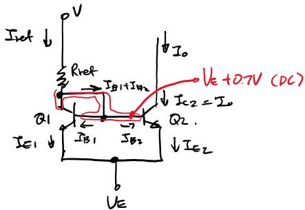
$$\text{Ohm's law: } I_{\text{ref}} = \frac{V - (V_E + V_{BE})}{R_{\text{ref}}}$$
