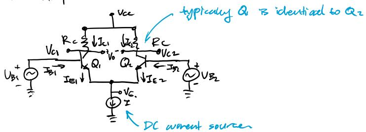
If  $V_{B1} = V_{B2}$ , then  $V_{BE1} = V_{BE2}$ , thus  $i_{E1} = i_{E2} = I_{E1} = I_{E2} = I/2$
