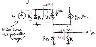
$$\tilde{U}_{b2} = \frac{V_{\pi 2}}{U_{b2}} = \frac{V_{01}}{U_{01}}$$
